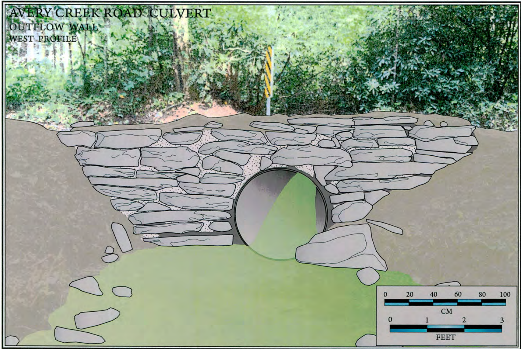
Figure 21. West profile drawing of outflow wall at Avery Creek Road culvert on FSR 477.
