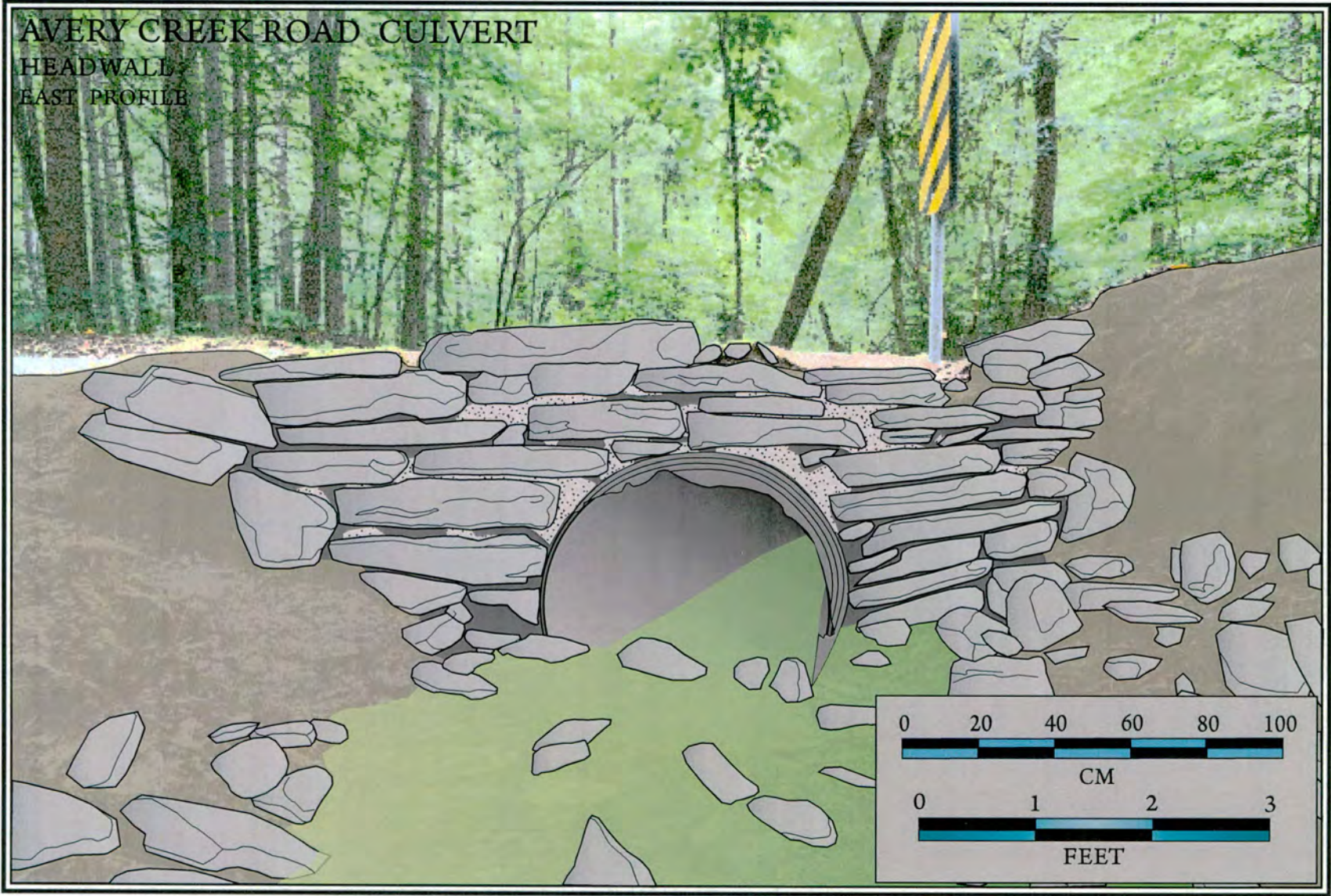
Figure 18. East profile drawing of headwall at Avery Creek Road culvert on FSR 477.
